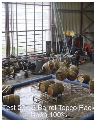
2 Barrel Steel Rack Fails 100% of the Napa quake simulation.
